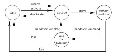
Figure 7.6: State machine for the distinguished MS behaviour
